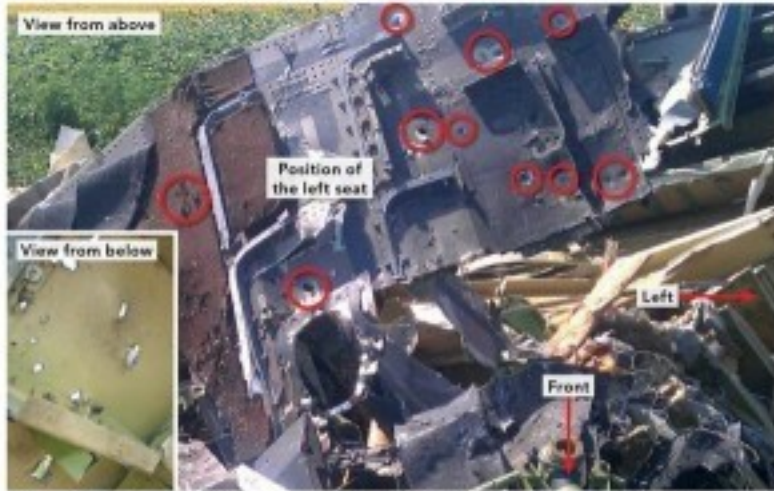
Figure 10: Cockpit floor with floor parts showing puncture holes (red circles) coming from above the floor. (Source: N844)
