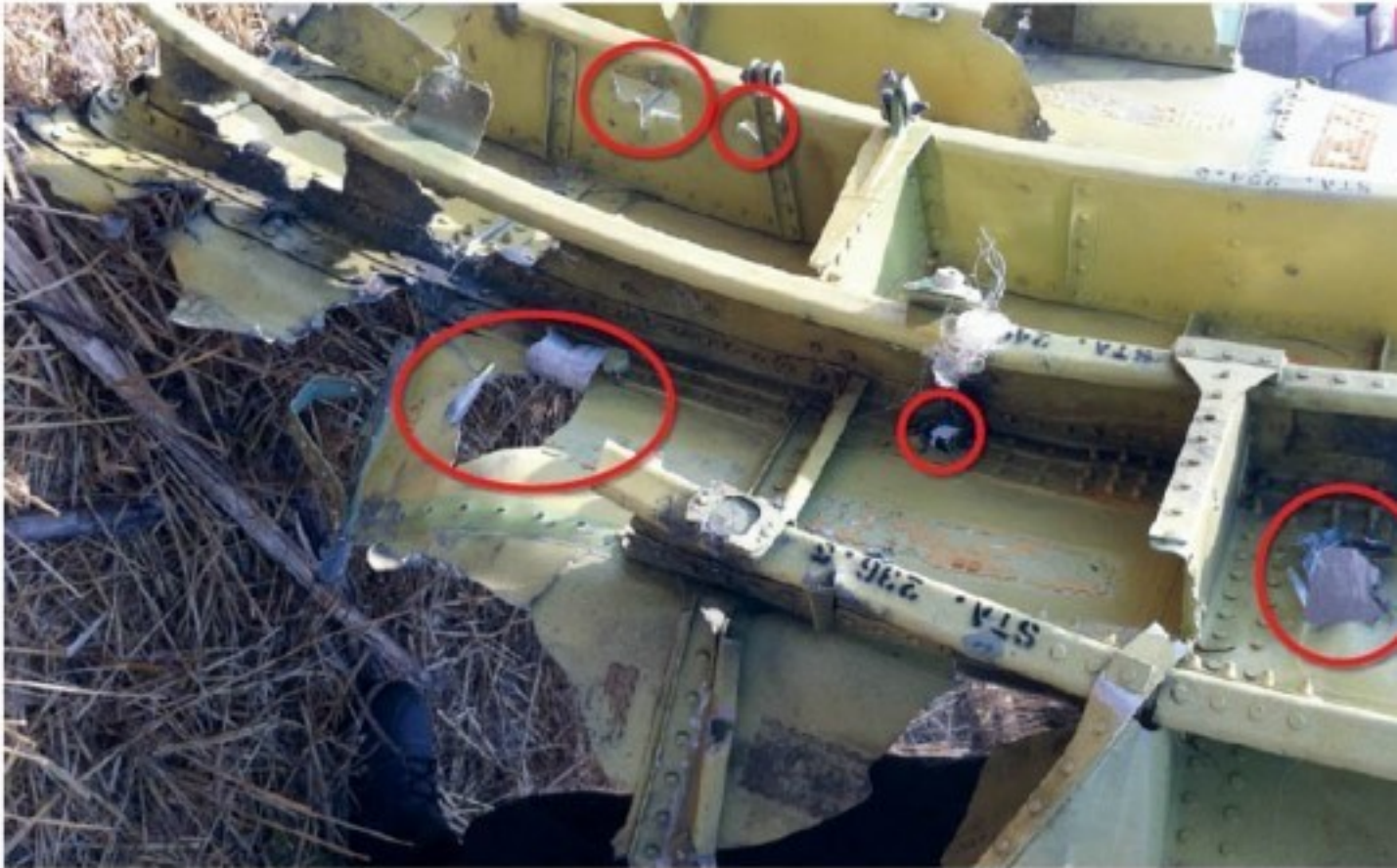
Figure 9: Part of the inside cockpit roof, indicating penetration with objects from outside. (Source: D
