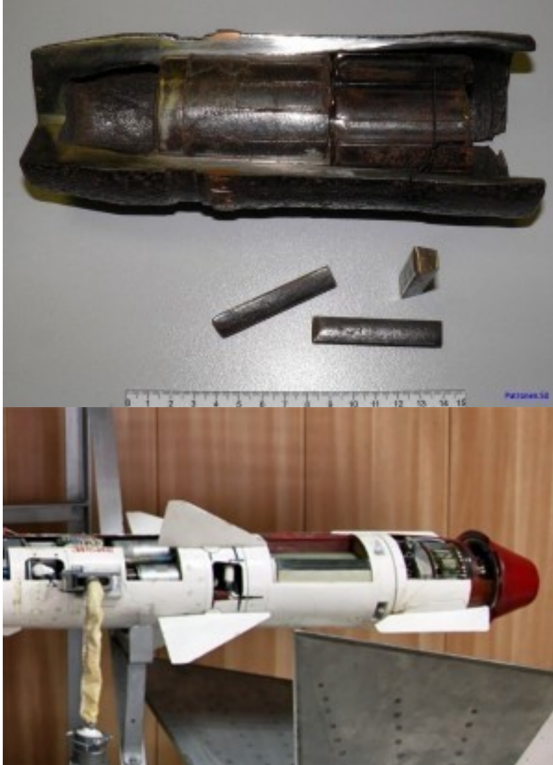
Left – this is approximately how the rod-based warhead that is used on the Ukrainian attack jets looks like ( Source ). Right – the warhead of the R-60 missile
