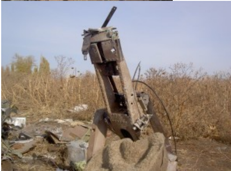
The back of the seat of the second pilot, numerous holes can be seen on the side and in the back.
